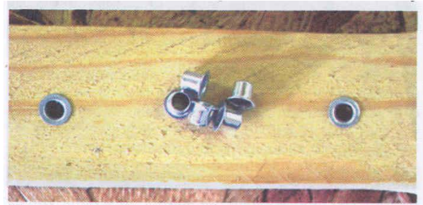
Two eyelets installed in an end bar.
